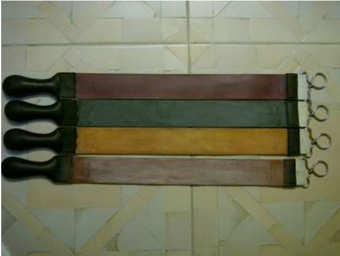
Strops, some different abrasive pastes (plain, chrome oxide, diamond, titanium oxide)
