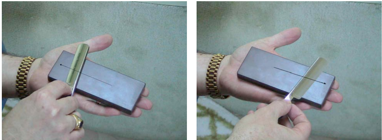
Honing on a Swaty, leading with the edge, and a very light touch!
