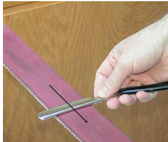
Stropping on the linen and leather sides of a hanging strop.
