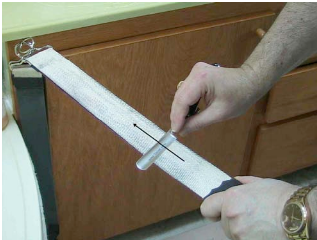
Stropping on the linen and leather sides of a hanging strop.
